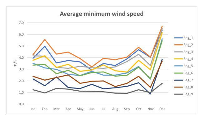
Figure 4-2: Average minimum wind speed per region for DLR calculation. Source: author. Data from European Centre for Medium-Range Weather Forecasts, 2017
