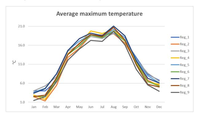
Figure 4-1: Average maximum temperatures per region for DLR calculation. Source: author. Data from European Centre for Medium-Range Weather Forecasts, 2017
